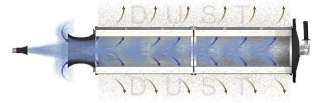
At any point along the cartridge filter, the VIPL unit provides 25% or more pulse cleaning power than the competition.
